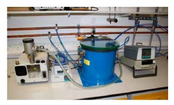
The rig has been designed specifically with commercial modules in mind – those measuring 40 x 40mm or 47 x 47mm can be fully characterised from room temperature to 200°C.
